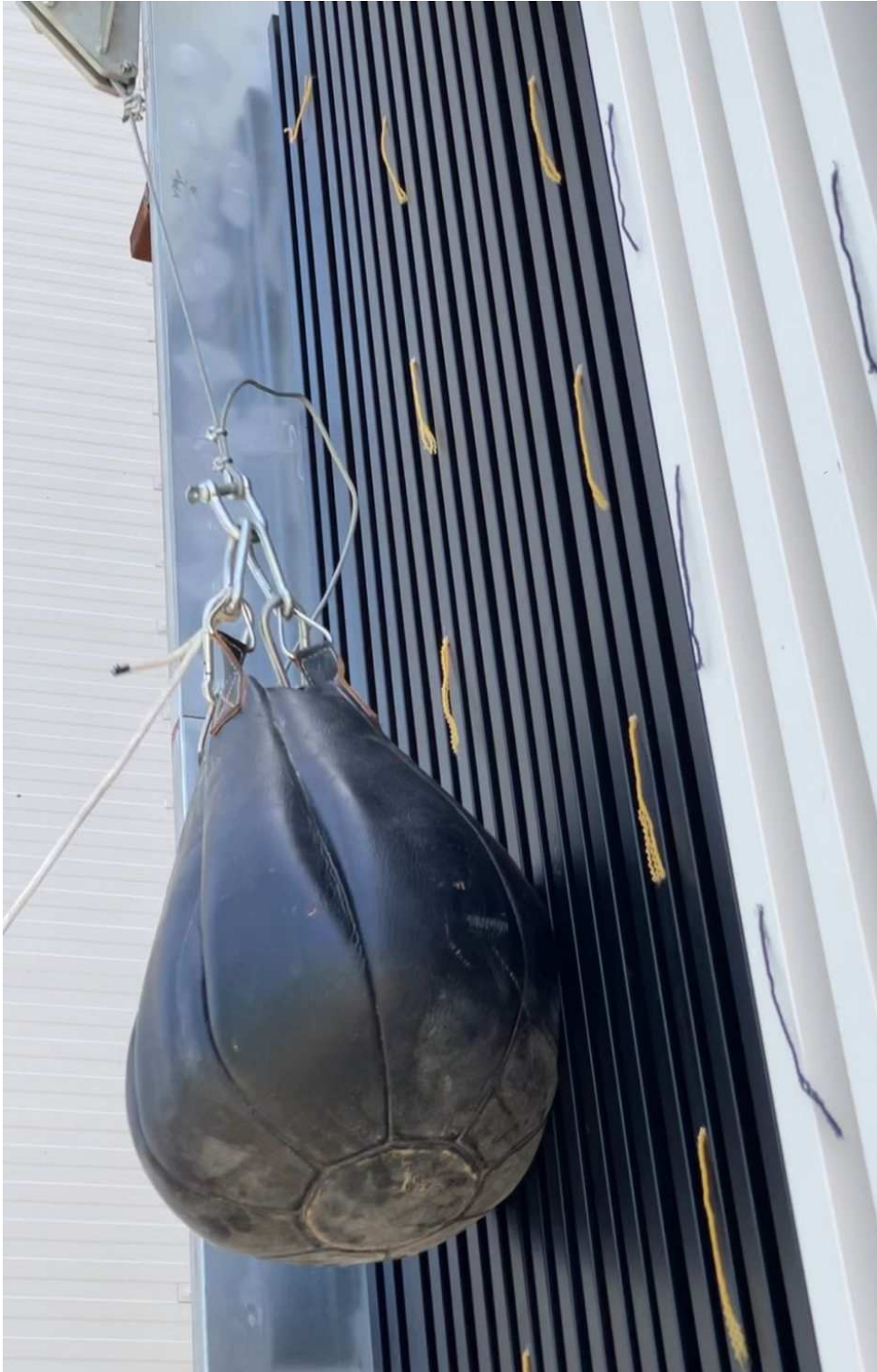
Foto 4. Test sample undergoing impact resistance with soft body_BATTENS 30
