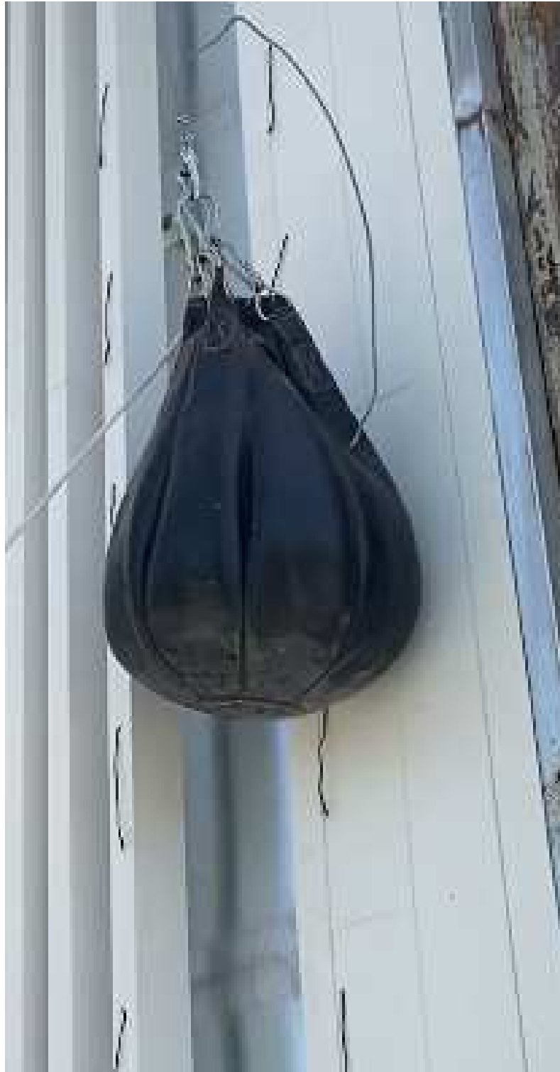
Foto 6. Test sample undergoing impact resistance with soft body _CLADDING 150
