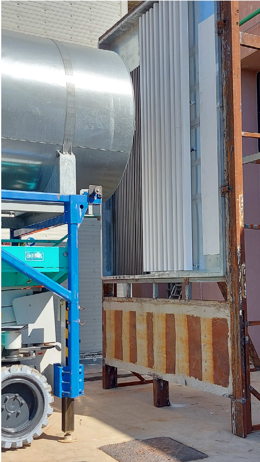
Foto 2. Tested sample undergoing resistance to wind load under dynamic pressures – orthogonal flow
