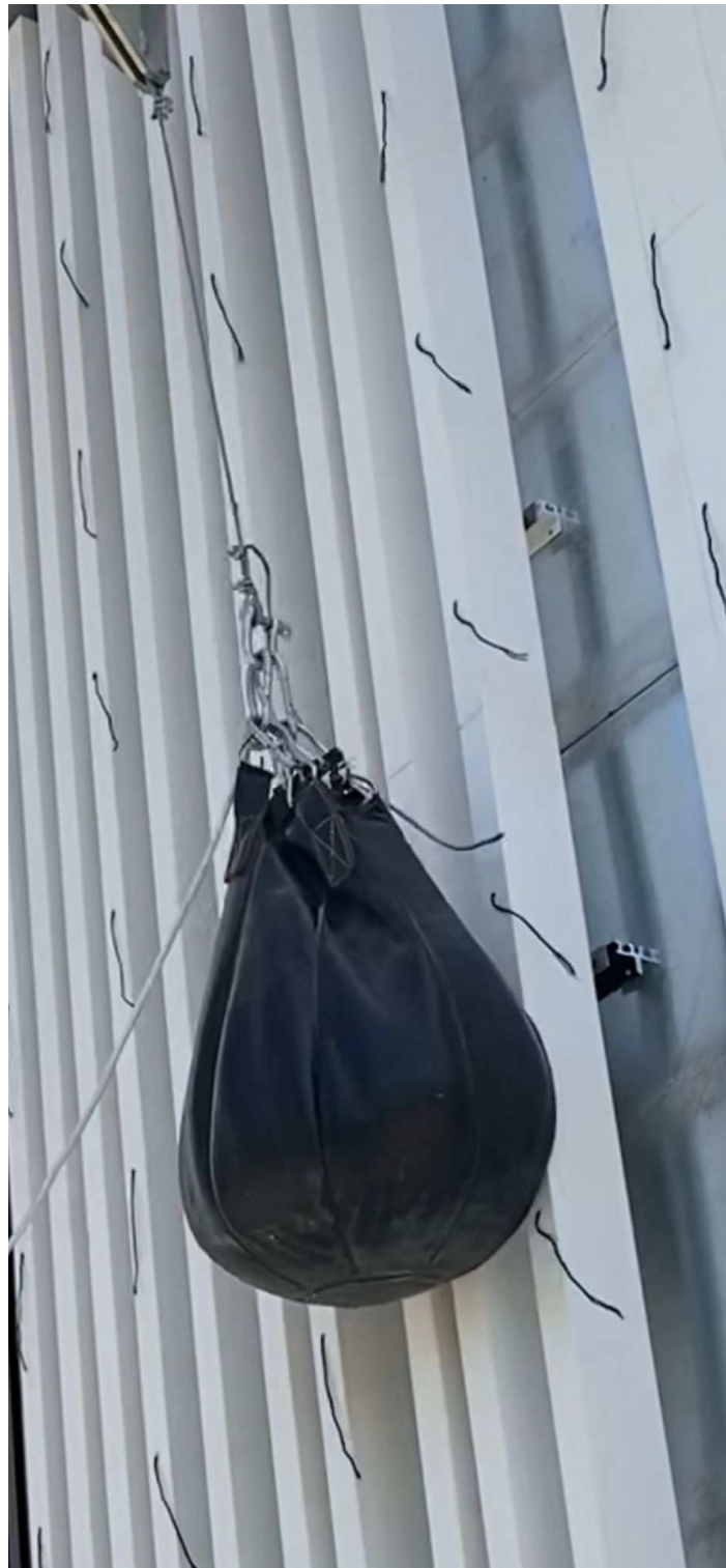
Foto 5. Test sample undergoing impact resistance with soft body _BATTENS 50
