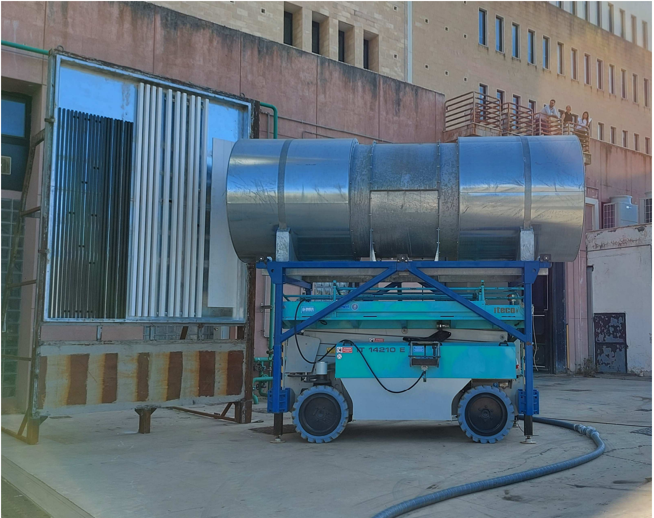
Foto 3. Tested sample undergoing resistance to wind load under dynamic pressures – air flow iclinated to 45°
